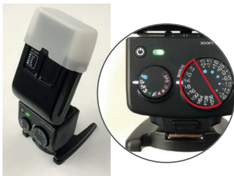
In the SF mode of the Nissin Digital i40, the light intensity can be manually adjusted using this dial.
