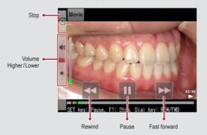
Movies can be operated by pressing the camera buttons or by rotating the dial key.
