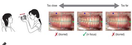
Do not press the shutter button until the distance is determined.
