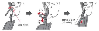
Put the other end of the strap through the strap eyelet. Adjust the strap while holding the camera until the optimal fit is obtained.
